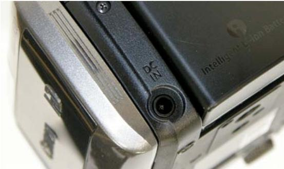
**Charging the battery and AC operation.** To charge the battery, plug the AC adapter into the DC IN socket on the back of the camera. The battery will only charge when the camcorder is turned off. The LED next to the power switch will flash red while the battery charges and stops when battery charging is complete. This camera may be powered using the AC adapter, however, the battery will not charge while the camera is turned on.
