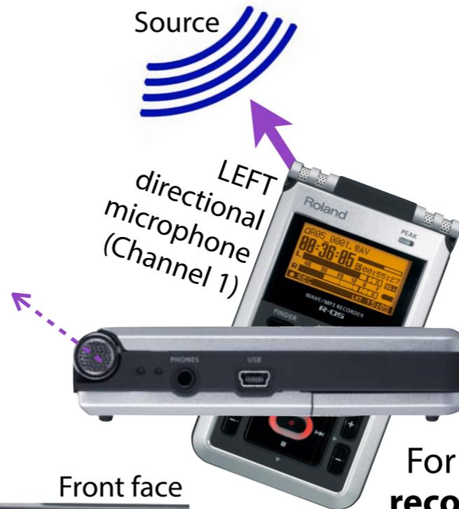
For the best quality **mono recording** into channel 1, point the left microphone towards the source (point the recorder about 60 degree angle towards the source and favoring the front face of the recorder)\*
