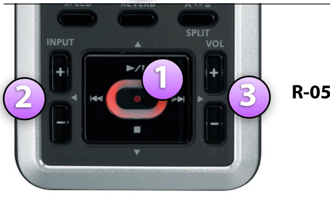
1. Press the ●REC button, the red ● flashes, indicating **Record-Standby** mode
