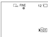
**5** Press PHOTO deeply. The image when you press PHOTO deeply is recorded on the "Memory Stick."
