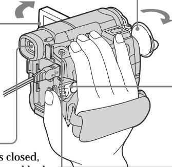
**2** Set the POWER switch to MEMORY while pressing the small green button. Make sure that the LOCK switch is set to the left (unlock) position.
