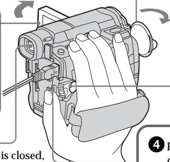
2 Set the POWER switch to CAMERA while pressing the small green button.
